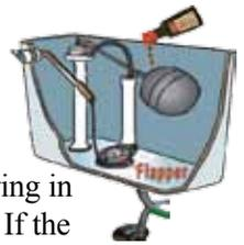
**1st** - put a couple of drops of food coloring in the tank and leave it for an hour or two. If the bowl water changes color the flapper needs to be replaced.
